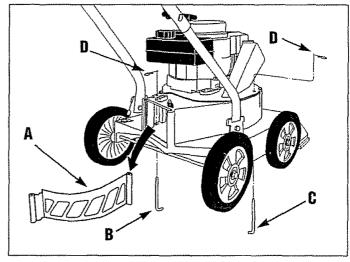
Figure 13: Shredder screen removal.
